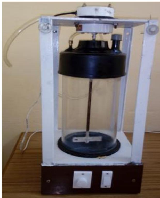
Fabricated pilot scale reactor
