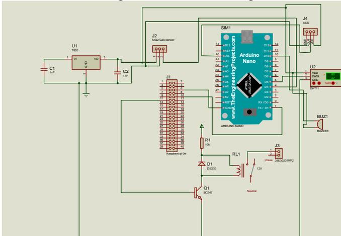
Fig 3.1 Circuit diagram of SRE
