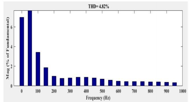
Fig. 5 a) Harmonics due to single EV connected at a charging station
