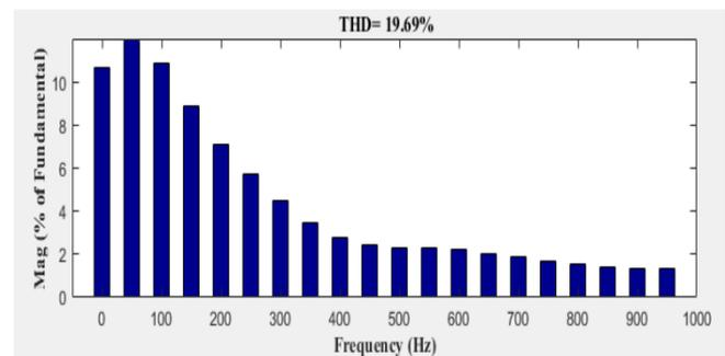
Fig. 5 c) Harmonics due to 5 EV chargers are connected at a charging station
