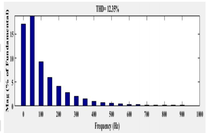
Fig. 5 b) Harmonics due to 3 EV chargers are connected at a charging station
