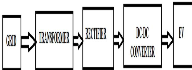
Fig.1: Block diagram of an EV Charging Station.
