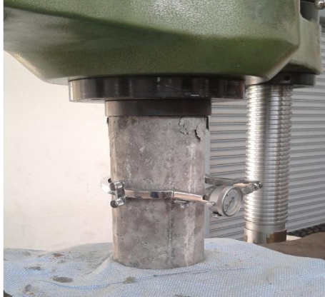
Fig 5 Compression test with longitudinal compressometer
