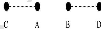
(Fig. 1) Neighboring nodes A and B have different schedules. They synchronize with nodes C and D respectively.
