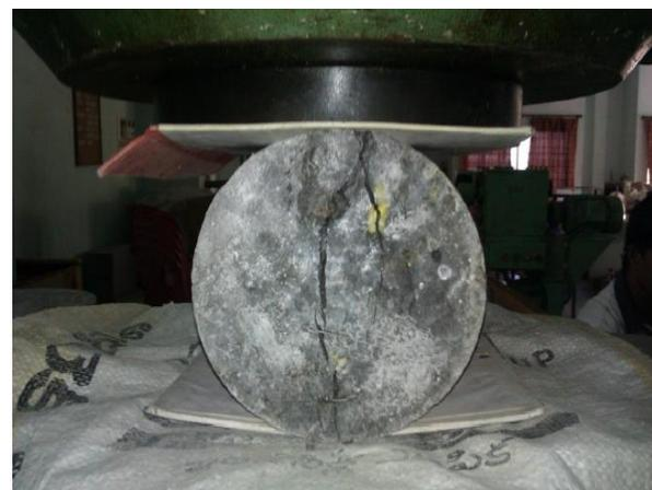
**Figure 2. Split Tensile Test**
