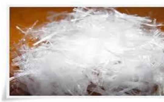
**Figure 1. Polypropylene Fibre**
