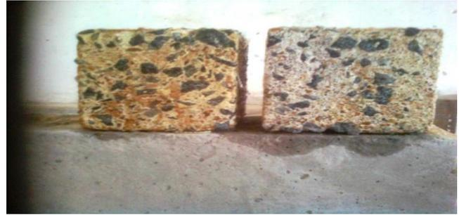
Figure 5 Polypropylene fibrous Concrete Cube after curing in H<sub>2</sub>SO<sub>4</sub>
