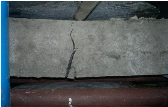
Figure 3. Flexural testing for Beam
