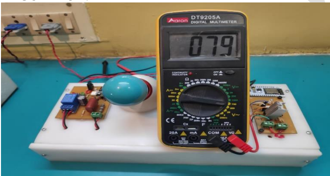
FIG 8.2 Display View Of Smart Switch And Smart Voltage Regulator
