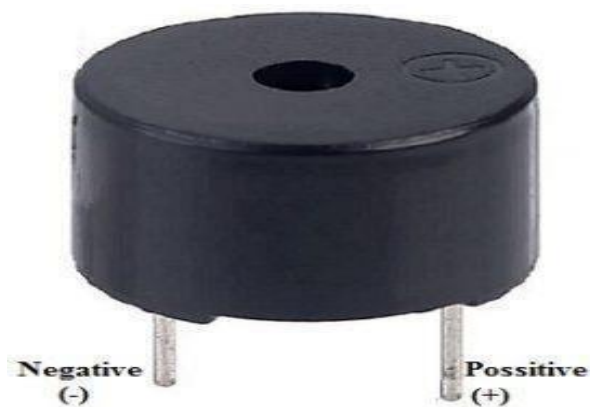
Fig. No 7 Buzzer Pin Configuration
