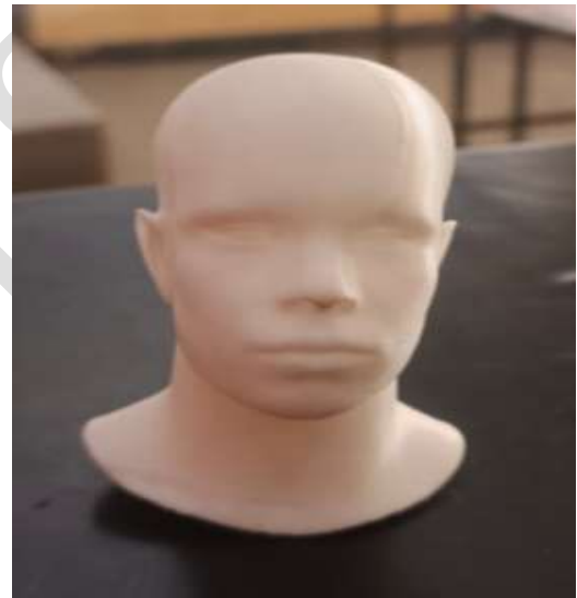
Fig.7Physical model fabricated in FDM
