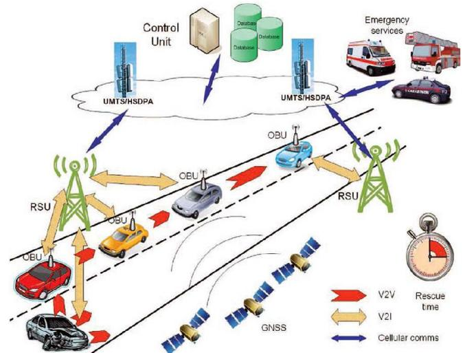
**Fig 1 Architecture of our proposed system for automatic accident**
