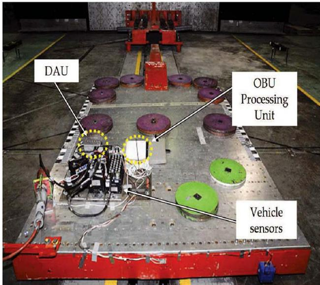
Fig 4 Sled with the prototype installed before a crash detection test.
