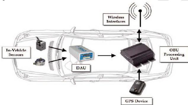
**Fig. 2. On-board unit structure diagram.**
