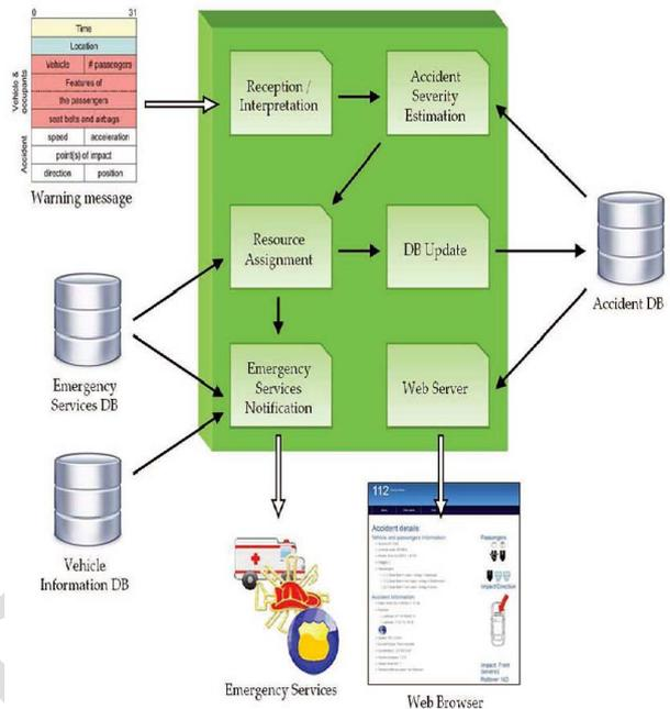
**Fig. 3. Control unit modular structure.**
